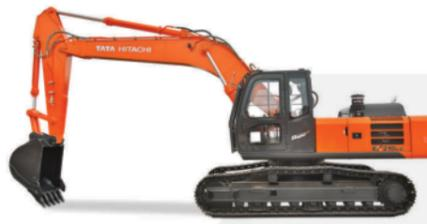
With factory fitted rock breaker piping kit as option
